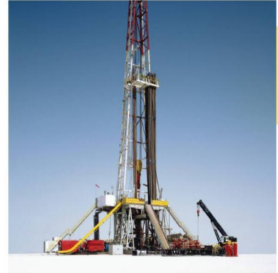
The string of drill pipe stacked on this oil rig will be subjected to extremely large axial deformations when it is placed in the hole.
